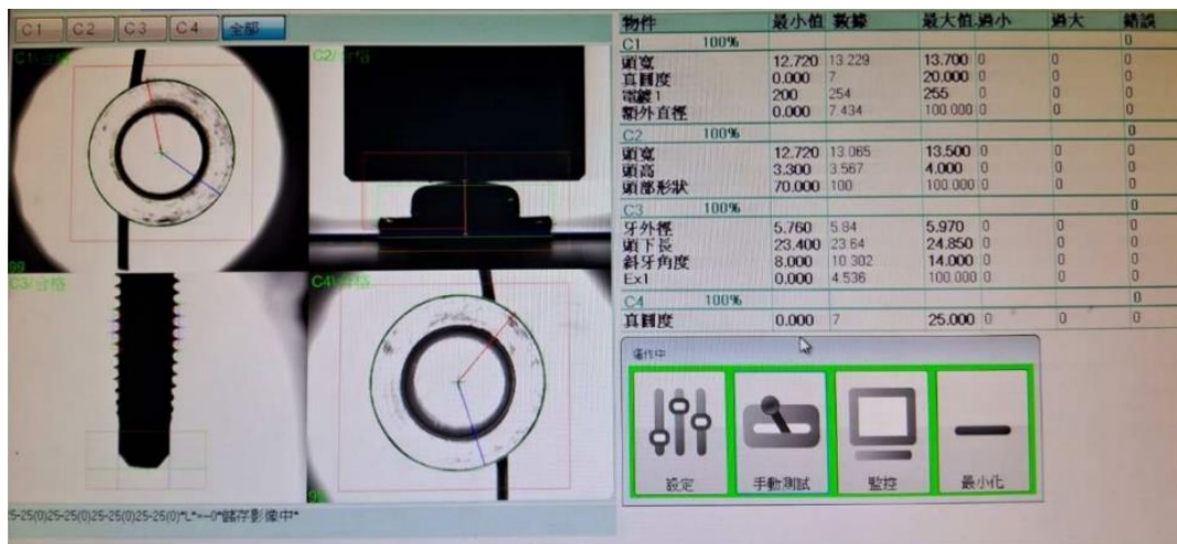
Fig.1 actual measurement screenshot of optical inspection with machine vision
