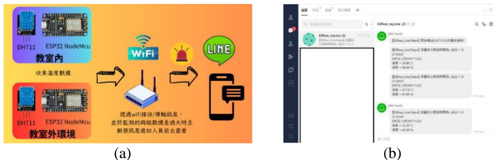
Fig.1 The architecture system diagram and output information
